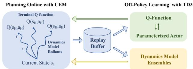
Figure 1. Overview: We use online planning with learned dynamic models and a terminal Q-function as the behavior policy. The transitions are saved into the replay buffer to train the Q-function and the dynamics model. The parameterized actor is also used to guide online planning.
