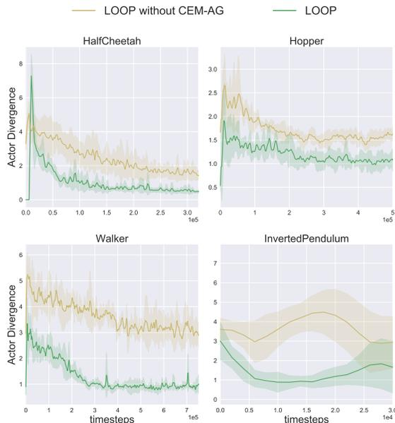
Figure 3. Actor-guided CEM reduces actor-divergence between the MPC policy and the model-free actor.
