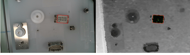
Figure 4. Robot view through a RealSense D435 camera, mounted to the robot arm. The depth image is binarized with a tuned threshold and contours are extracted. A rectangular bounding box (red) is drawn for contours of the expected size and used to calculate an aligned and centered grasp. Averaging the calculated grasps over multiple frames improved the stability, resulting in 100 consecutive successful grasps when only a single object is in frame.
